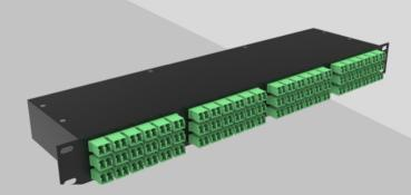
A cost effective pre-terminated MTP® solution for quick deployments. Enclosure is pre-terminated with MTP® pinned connectors in the back, and LC connectors on the front. The most common units feature 12 fiber MTP® connectors routed to 6 duplex LC on the front. Mix and match single and multimode fiber types per set of 12 LC fibers, or mix and match fiber types per MTP® connector.
